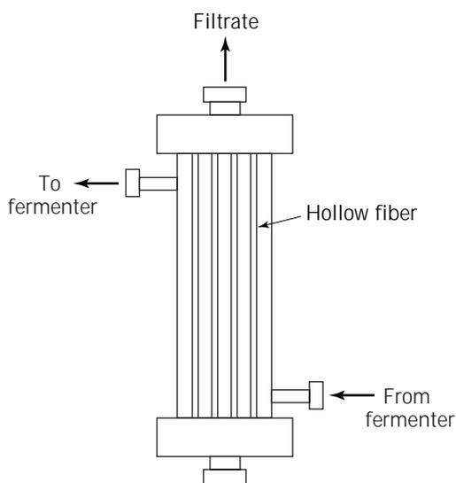
**Figure 4.** Schematic presentation of the hollow-fiber modules for sampling. A perfusion buffer is passed through the lumen of the fibers, and the fermentation broth is introduced on the shell side of the unit.
