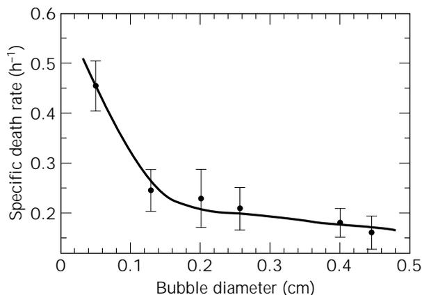
**Figure 8.** Effect of bubble diameter on the specific death rate of *S. frugiperda* insect cells in bubble columns aerated at a constant volumetric gas flow rate of 10 mL min<sup>-1</sup>. Source: Adapted from Ref. 113.
