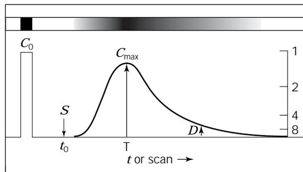
**Figure 9.** In addition to peak height a dispersed sample zone yields an infinite number of vertical readouts. The initial concentration,  $C_0$ , is injected at time  $t_0$ , and the pulse appears as a continuum of concentrations as exemplified by the peak. At time  $T$ ,  $C_{max}$  is the highest value read, but a reading could be done anywhere along the peak (e.g., a diluted value at point D).
