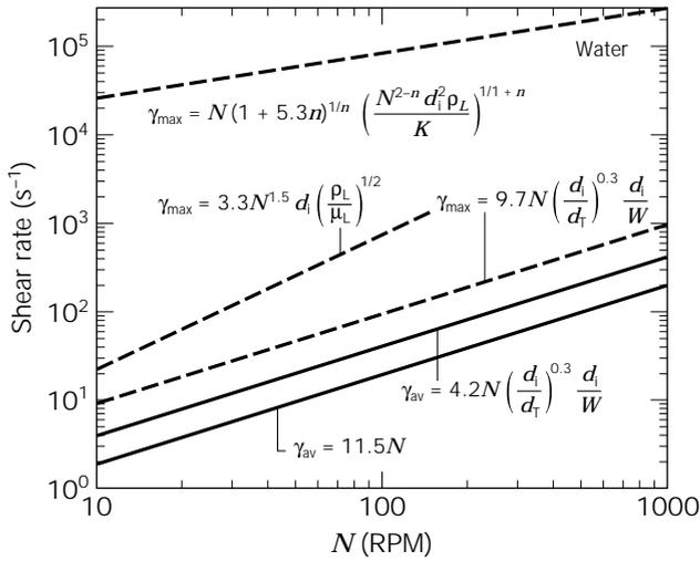
**Figure 2.** Comparison of the various shear rate correlations for water in a standard stirred-tank agitated with a 0.1-m-diameter six-bladed Rushton turbine. The dashed lines are for the maximum shear rate; the solid ones are for the average shear rate. See text for additional details.
