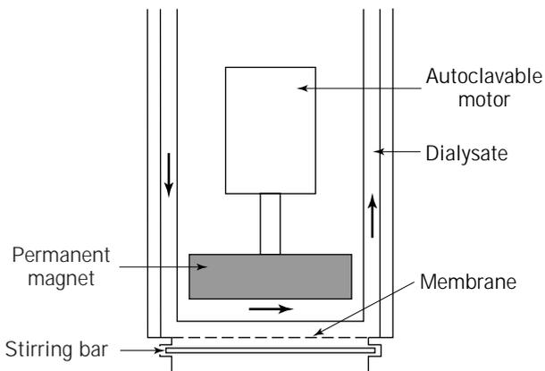
**Figure 5.** Cross section of the dialysis probe. The stirring bar is rotated by the rotating magnetic field when the motor is on. Receiving solution is pumped over the inner side of the membrane where dialysate is received and removed for analysis. *Source:* From Ref. 48.
