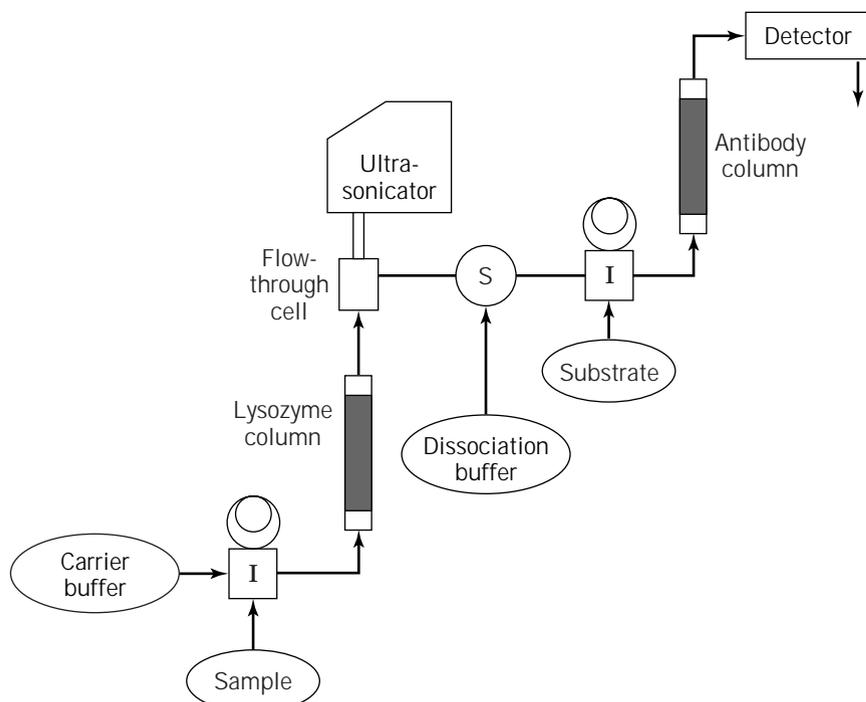
**Figure 7.** Schematic presentation of a complete flow system, including an expanded flow column with immobilized lysozyme and ultra-sonicator flow cell. An expanded column with immobilized antibodies is also included for the subsequent ELISA.
