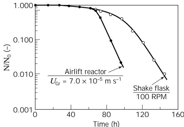
**Figure 6.** Survival of suspended porcine erythrocytes in a sparged airlift bioreactor and a surface aerated shake flask. Normalized cell count ( $N/N_0$ ) is plotted as a function of time. Source: From Ref. 43.
