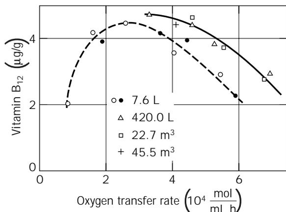
**Figure 20.** Production of vitamin B<sub>12</sub> as function of the oxygen transfer rate.
