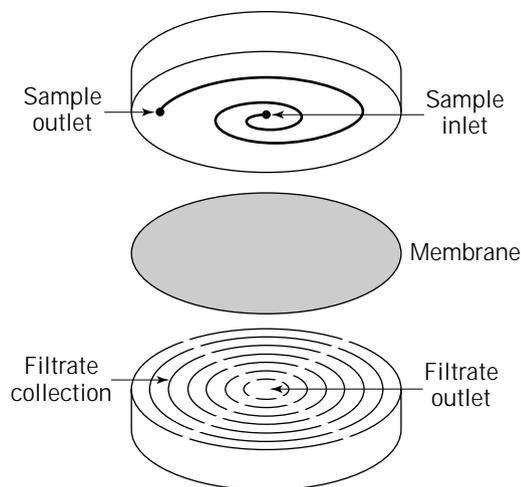
**Figure 3.** Schematic presentation of the flux membrane dialysis module. The membrane is mounted between the two holders, and sample is introduced on one side. The filtrate is collected and transported for future analysis.
