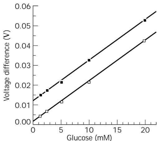
**Figure 11.** On-line outlet signal (V) as a function of glucose concentrations (mM); (■) glucose standard solution with added internal standard (5 mM),  $y = 1.14 \times 10^{-2} + 2.05 \times 10^{-3} x$ ,  $r^2 = 1.000$ ; (□) glucose standard solution,  $y = 1.09 \times 10^{-2} + 2.04 \times 10^{-3} x$ ,  $r^2 = 1.000$ .
