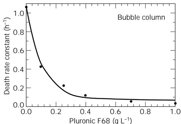
**Figure 12.** Cell protective effect of Pluronic® F68 in a bubble column. The specific first-order cell death rate constant is plotted as a function of the concentration of Pluronic F68 in the medium. All data were obtained at a constant specific power input of  $\sim 40\text{ W m}^{-3}$ . Source: Adapted from Ref. 112.
