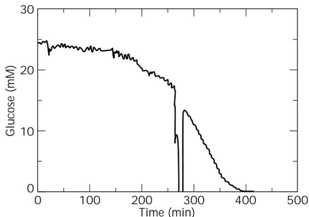
**Figure 10.** Monitoring of glucose in batch cultivation of *Escherichia coli*. After approx. 270 min a calibration solution is introduced, and the reading is back approx. 10 min later. Source: From Ref. 20.
